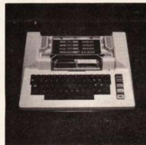
Atari 800 Console (with cover removed)
